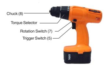
The item numbers (in brackets) can be found on the Drill Assembly and Drill Parts List.
